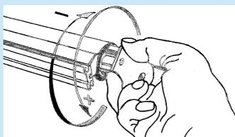
Relocate the new spring unit leaving the head projecting about 20mm and place the end bracket back onto the spring end. Turn the bracket anti-clockwise approximately 10 – 14 turns depending on the width of the blind. Push the spring and end bracket back into the roller tube locating the bracket lugs in the fitting rail at the same time. Secure back with the screw. Test the blind for tension and if necessary increase or decrease using the adjusting screw in the end bracket.
