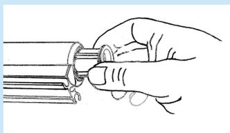
Withdraw the spring unit. You may need a small flat bladed screwdriver to ease out the first few millimetres.
