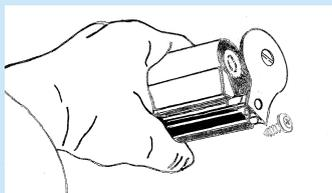
Take out the screw that retains the end cap to the fitting rail and prise the end cap off gently.
